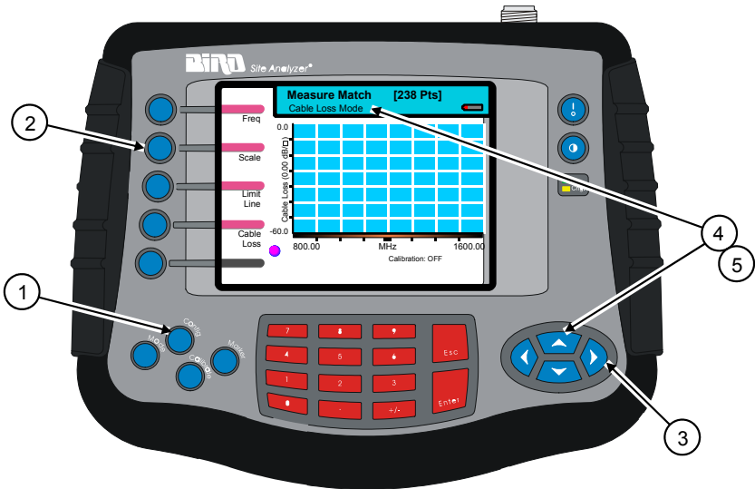
Figure 18 Set Up for Cable Loss Measurement
