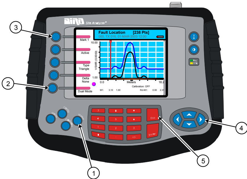
Figure 37 Using Markers with Recalled Traces
